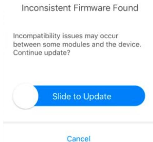
To update the firmware of your TB60 batteries (used with the M300 RTK), place them in the BS60 Battery Station and connect the Smart Controller Enterprise to the battery station. Multiple batteries can be updated at once in the health management system of the Pilot App.
