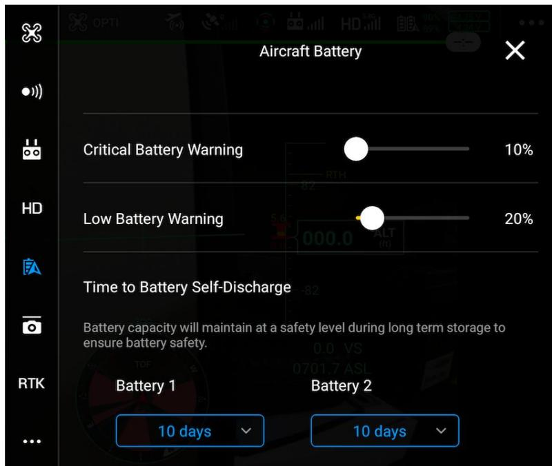
For users who require batteries to always be at 100%, it must be understood that this will negatively affect the life and performance of lithium-ion batteries. When a battery is at 100% it places stress onto the cells and leaving that stress on the cells will accelerate a decrease in the batteries' capacity and operational life cycle.
